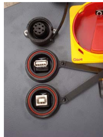
Figure 3c: connectors detail (USB for BEAT HF-Tr only)
