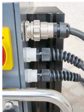
Figure 11a: Mains cable (plugged)
