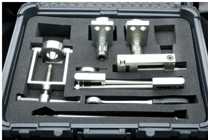
Set of drilling machine with accessories inside the transport casing
